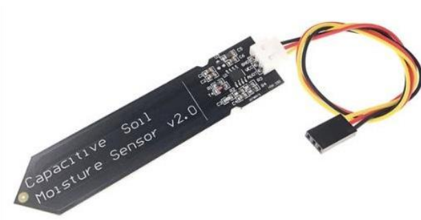
Figure 7. Design of soil moisture sensor on IoT
