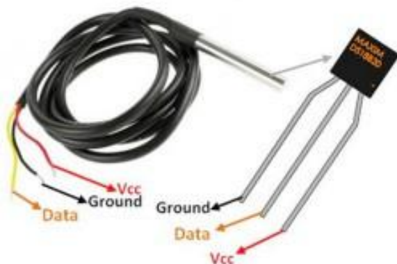
Figure 5. Design of water temperature sensor on IoT
